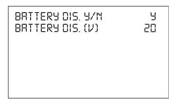
**BATTERY DISCONNECT Y/N**: Battery Disconnect active/passive **BATTERY DISCONNECT(V)**: Battery Disconnect voltage level
