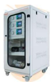
ASC ATU MULTI RACK is a switching unit for any MV Switching Centers needs redundancy and required chargers work in parallel. In case of any failure in a charger, ASC ATU automatically switches to the 2nd charger and let the system continue working properly.
