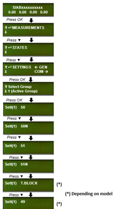
From the standby mode screen, press the “OK” key to access the first line of menus.
