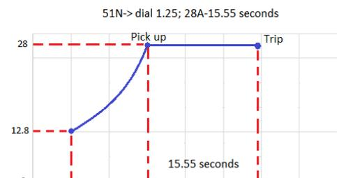
Note: In TEST 2 and TEST 3 for 51 and 51N, the fault current will be injected directly to check the theoretical tripping time. Take into account that this time is calculated through an equation and this time depends on the injected current. In doing this, a ramp is possible but the theoretical tripping time will not be checked.
