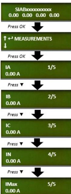
From the standby mode screen, press the “OK” key to access the first line of menus.
