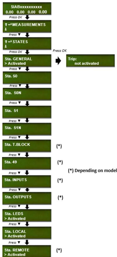
The States menu indicates the status of the relay (activated or deactivated) on real time.
